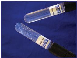
BTI's unique neutron **bubble detectors** are the world's most sensitive and accurate neutron dosimeters. They have been used by nuclear facilities, hospitals, military groups, and space agencies for neutron measurements and **personal neutron dosimetry** for over twenty-five years.
