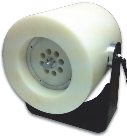
The Neutron Long Counter is an important tool for fast-neutron measurements. As a result of its sophisticated internal structure, it has a nearly flat (+/- 15%) efficiency as a function of neutron energy from ~150 keV to > 15 MeV. Thus relative neutron output of various neutron sources can be quite accurately measured independent of source type. This is in stark contrast with the order-of-magnitude efficiency variation over the same energy range for simpler spherical-moderator-type systems.
